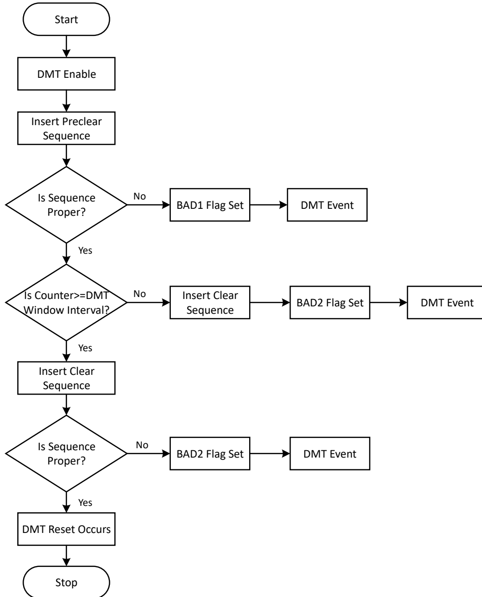
Figure 20-2. Flowchart for Clearing the DMT
